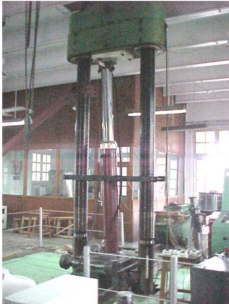
Fig. 1: 600 Tonne leg testing machine approved by DGMS
