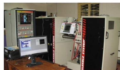
Thermo-Mechanical Simulator (Gleeble 3800)
