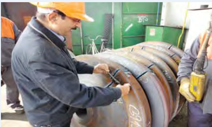
Inspection of Loco Wheel Disc at Czech Republic
