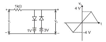
Assuming the diodes to be ideal, which of the following graphs depicts the output voltage  $v_0$  as function of time t ?
