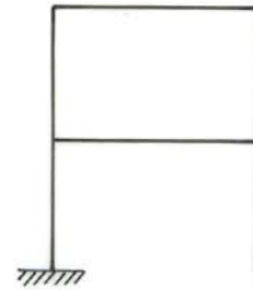
FIG. 5-2. EXTERNALLY DETERMINATE BUT INTERNALLY INDETERMINATE PLANE SYSTEM
