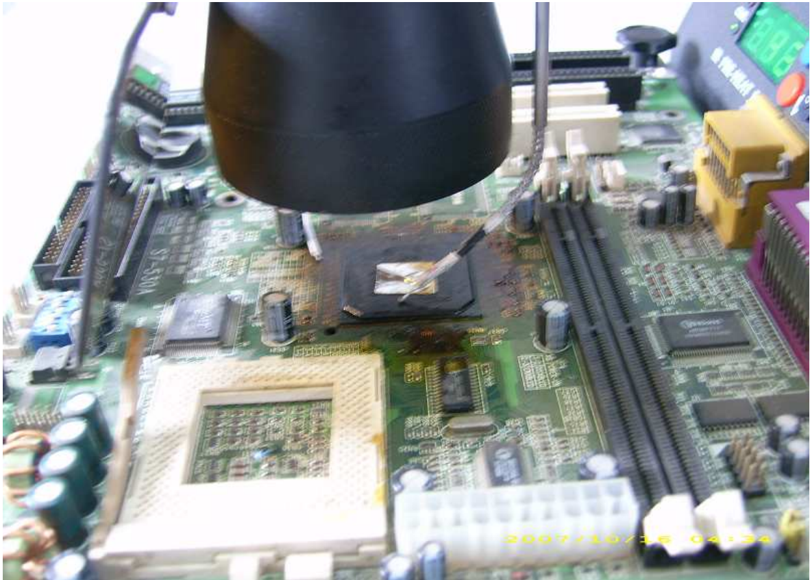
(The position of the two Temp-sensor when soldering the south/north board)
