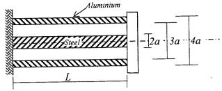
aluminium tube. Use G for rigidity modulus for steel and 0.5G for aluminium.
