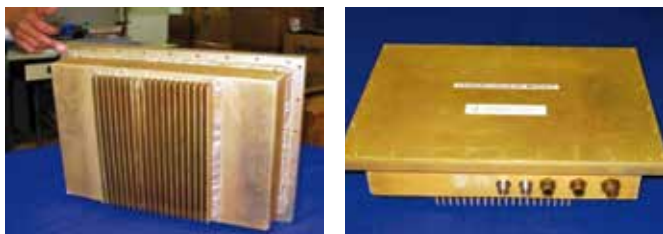
T/R module for ST Radar
