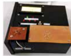
Handheld electronic for gas sensor power and readout MEMS gas sensor capped with perforated metal cap.
