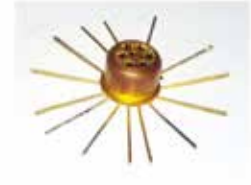
Handheld electronic for gas sensor power and readout MEMS gas sensor capped with perforated metal cap.
