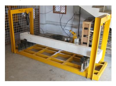
Fig. 3.10 Torsion Testing Equipment
