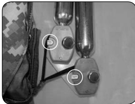
7.1.6 Installing the green safety clips.
