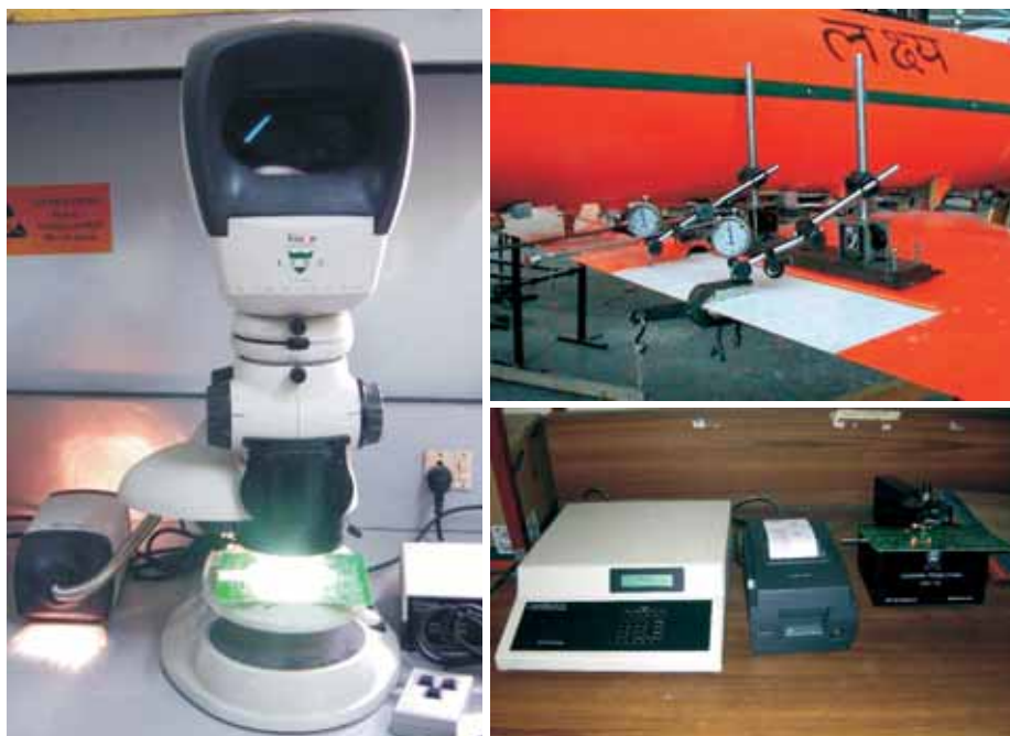
Optical zoom instrument for inspection of PCBs (left). Actuator stiffness test (top) and copper thickness measuring instruments for PTH and surface PCBs.
