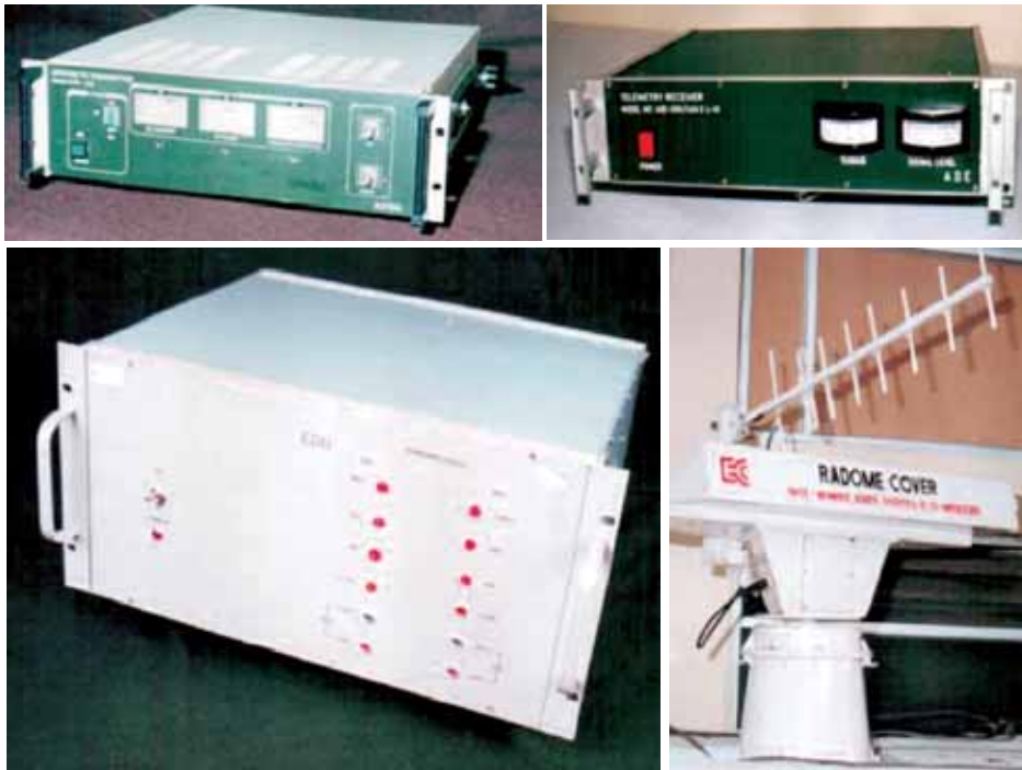
Radio frequency packages (clockwise from top right): Receiver; antenna with tracking mechanism; encoder-decoder unit; and transmitter.
