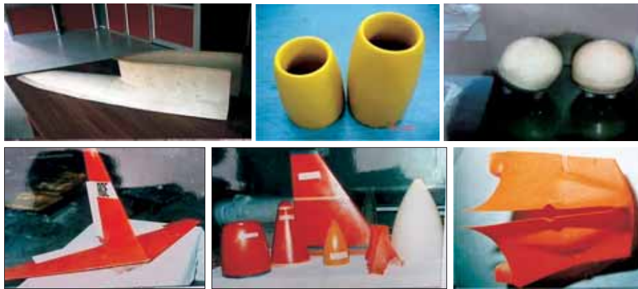
Composite technologies (from extreme left top): PTA fairing (front); air-in-take; Luneberg lens; tail fin assembly; different composite parts; PTA fairing (rear).
