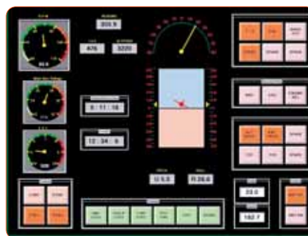
Ground control system displays UAV's flight path and parameters.
