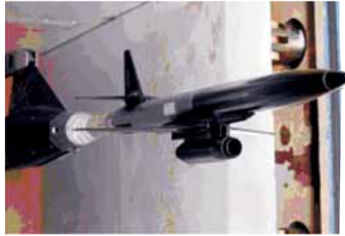
Wind tunnel testing of Lakshya.
