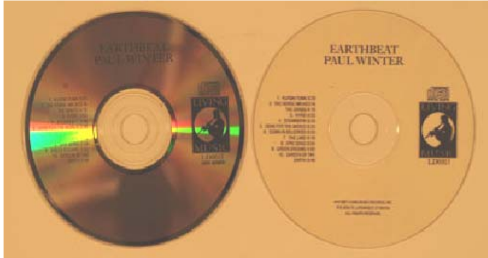
Image 4. Two CDs after 500 Hours of accelerated aging
