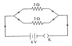
The current flowing through each of the resistors connected in the above circuit is
