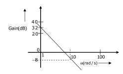
The gain  $(20 \log |G(s)|)$  is 32 dB and -8 dB at 1 radians/s and 10 radians/s respectively. The phase is negative for all  $\omega$ . Then G(s) is
