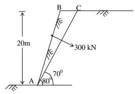
The factor of safety of slope when bolts are installed perpendicular to the failure plane is
