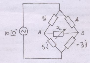
**Q8)** Find the R-L network corresponding to the driving point impedance using Cauer form I and Cauer form II.
