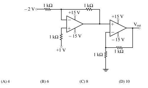
Q.30 In the circuit shown below the op-amps are ideal. Then  $V_{out}$  in Volts is
