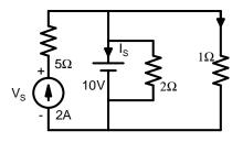
Q.48 The current  $I_s$  in Amps in the voltage source, and voltage  $V_s$  in Volts across the current source respectively, are
