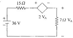
The power dissipated in the controlled source of the network shown above is
