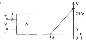
The voltage-current relationship feeding the network N is shown in the above figure. The Thevenin's equivalent of network N will have  $V_{Th}$  and  $R_{Th}$  as
