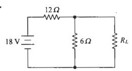
In the circuit shown above, the maximum power absorbed by the load resistance  $R_L$  is
