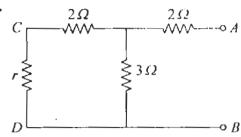
For the circuit shown above the value of r connected between C and D is such that the equivalent resistance of the circuit by looking into circuit through terminals A and B is r only. Then the value of r is
