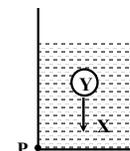
A sphere Y of mass  $M$  is falling with its terminal velocity in a viscous liquid X kept in a container.
