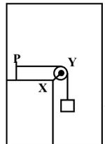
A pulley Y of mass  $m_0$  is fixed to a table through a clamp X. A block of mass  $M$  hangs from a string that goes over the pulley and is fixed at point P of the table. The whole system is kept in a lift that is going down with a constant velocity.
