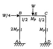
What is the bending moment at B at collapse conditions?
