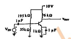
For the circuit shown above taking  $\beta = 200$  and  $V_{BE} = 0.6$  V
