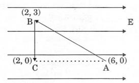
A test charge 'q' is moved without acceleration from A to C along the path from A to B and then from B to C in electric field E as shown in the figure. (i) Calculate the potential difference between A and C. (ii) At which point (of the two) is the electric potential more and why?
