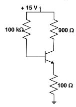
Which one of the following correctly represents the load line (collector current  $I_C$  with respect to collector-emitter voltage  $V_{CE}$ ) and Q-point of this circuit?
