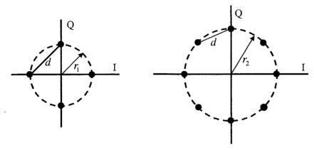
Q.52 For the constraint that the minimum distance between pairs of signal points be d for both constellations, the radii  $r_1$  and  $r_2$  of the circles are
