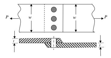
width of the plate w = 200 mm, thickness of the plate t = 5 mm, number of rivets n = 3, diameter of the rivet  $d_r = 10$  mm, diameter of the rivet hole  $d_h = 11$  mm, allowable tensile stress of the plate  $\sigma_p = 200$  MPa, allowable shear stress of the rivet  $\sigma_s = 100$  MPa and allowable bearing stress of the rivet  $\sigma_c = 150$  MPa.
